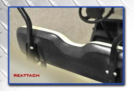
Reattach seatback using hardware from step 2.
