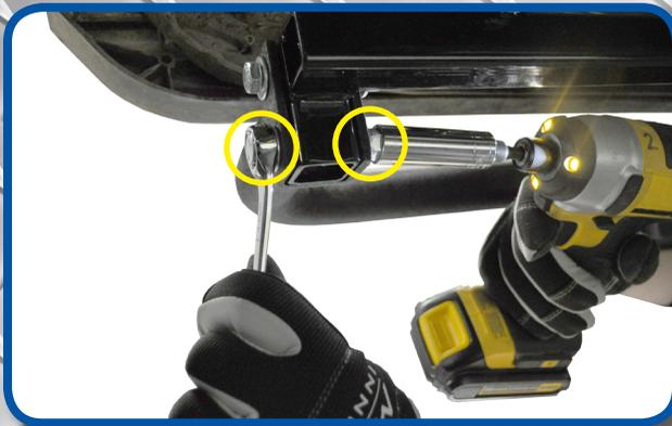
Using the 10mm x 55mm hardware provided attach step to bracket using 17mm socket and wrench. Once all 4-bolts are in place then tighten.
