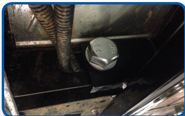
Secure bracket in both mounting locations using 20mm hardware provided. Tighten bracket hardware.
