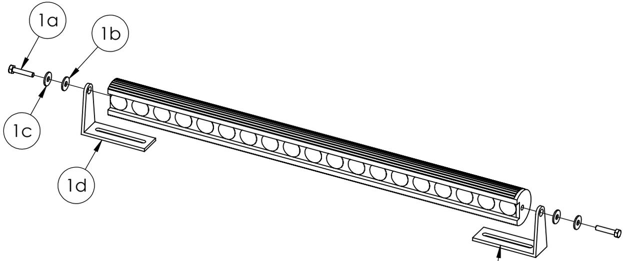
Brackets can be installed facing the opposite direction as well
